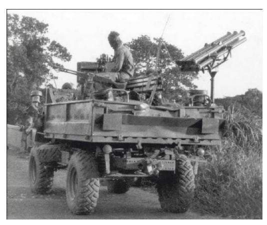
Unimog with home-made mounted SNEB (white phosphorus) and armour-piercing rocket launcher.
