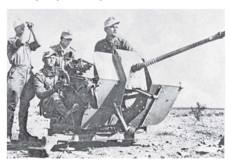
A 20-mm *Flak 38* antiaircraft gun, here in use in the ground combat role. Note the white "kill rings" on the barrel.
