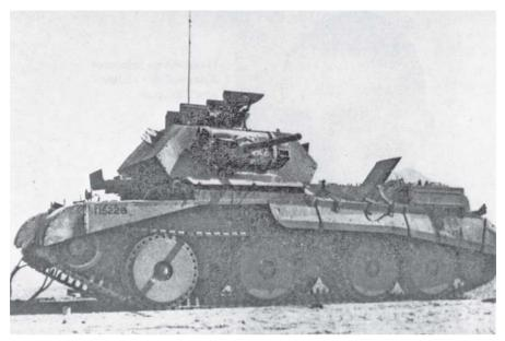
A destroyed British Crusader tank. Great things were expected of this vehicle but it was a disappointment, being mechanically unreliable and still mounting the inadequate 2-pounder main gun.
