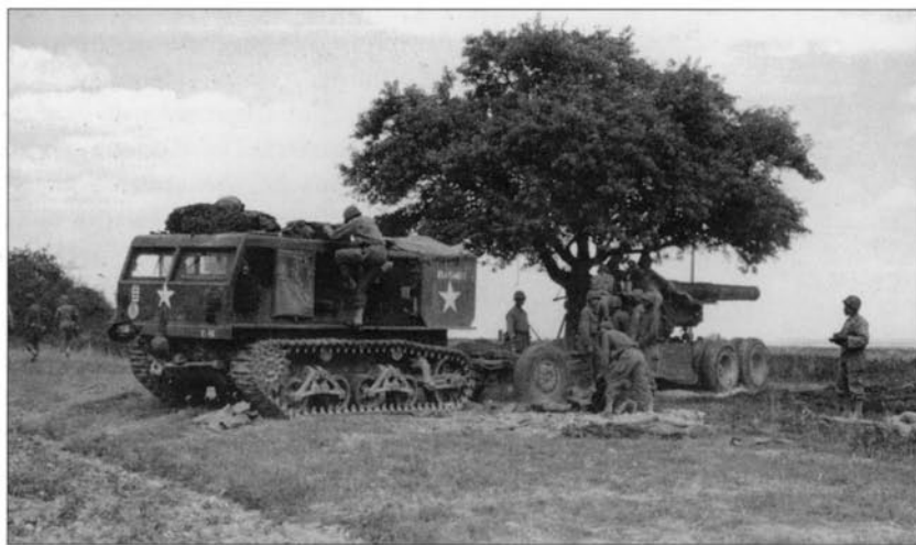
The US Army had a significant advantage over the Wehrmacht in artillery, both in terms of quantity and quality. US heavy artillery was mechanized, using fully tracked tractors like this M4 high speed tractor towing an 8-in. howitzer of the 999th Field Artillery Battalion (Colored) near Nantes-Gassicourt on 20 August 1944. (US Army)
