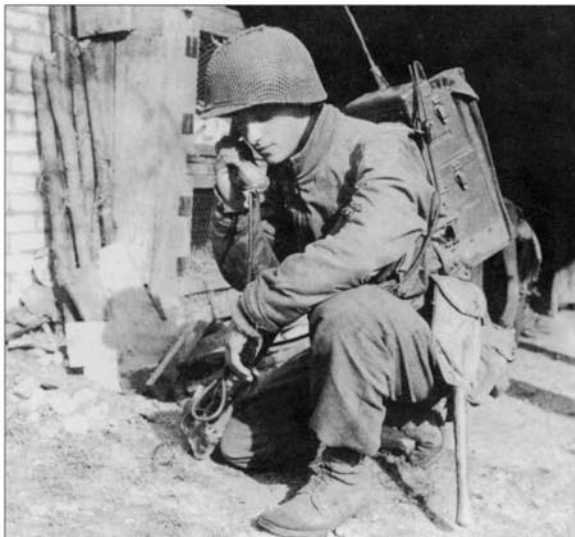
The US Army enjoyed advantages in communications, with more advanced equipment like the SCR-300 "walkie-talkie" radio. This was the first widely used FM infantry radio, and offered better performance than the German AM radios. It is seen here in use near Vagny, France, on 17 October 1944. (US Army)
