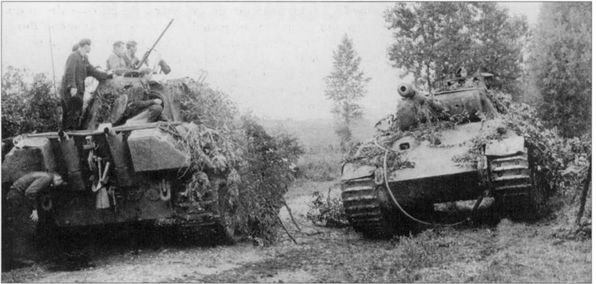
A pair of Panther Ausf. G tanks of Pz. Brig. 111 during operations near Parroy in late September 1944. It was a common practice at this stage of the war to cover the tanks heavily in foliage in an attempt to protect them from aircraft attack. (USNA)
