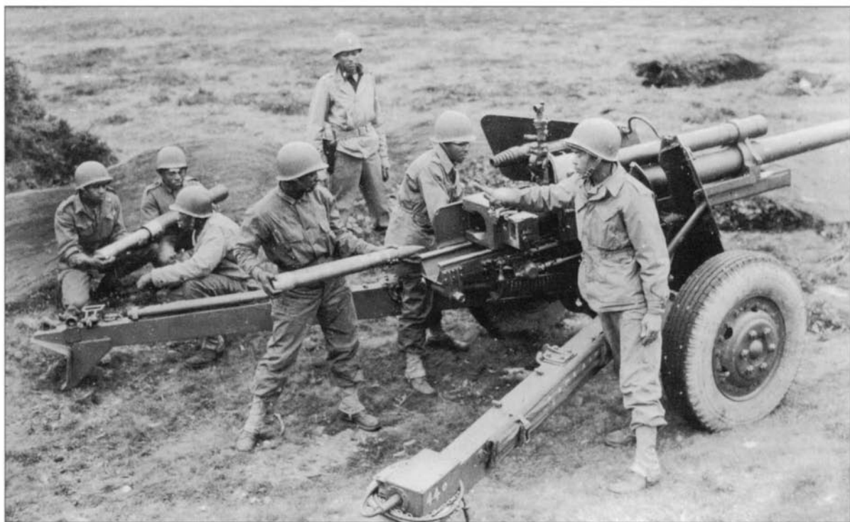
ABOVE The attack on Mairy was broken up with support from the 607th Tank Destroyer Battalion. This unit was equipped with the M6 3-in. anti-tank gun, as seen here during training exercises with the 614th Tank Destroyer Battalion (Colored) on 23 September. (US Army)
