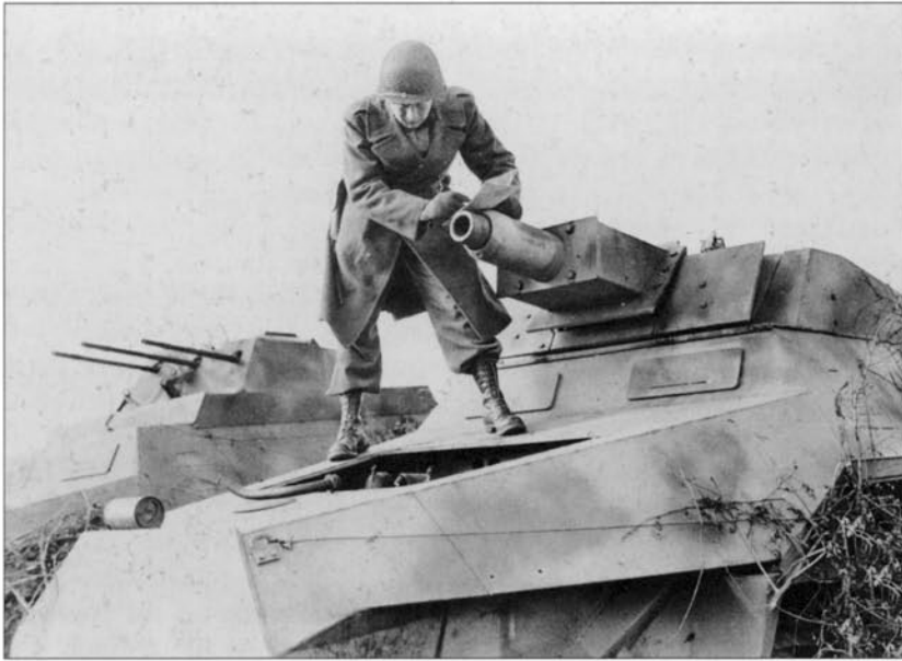
A GI from the 90th Inf. Div. inspects some of the German equipment captured by the division during the fighting with Pz. Brig. 106 near Mairy. These are both armed versions of the standard German Hanomag SdKfz 251 Ausf. D armored infantry half-track. An SdKfz 251/21 anti-aircraft vehicle with a triple MG151 30mm cannon mounting is seen to the left. Pz. Gren. Bn. 2106 had ten of the SdKfz 251/9 Stummel assault gun armed with a close support 75mm howitzer, seen on the right. (US Army)
