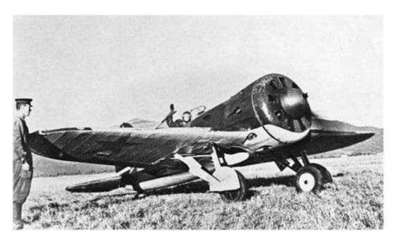
The world's first cantilever-winged monoplane fighter with retractable landing gear, Polikarpov's I-16 formed the backbone of the Soviet Air Force at the time Hitler's forces invaded Russia. Nicknamed Ishak ("Donkey") by its own pilots for the I-16's unpleasant, even potentially life-threatening flight characteristics, it was decimated in combat. (Courtesy Art-Tech)
