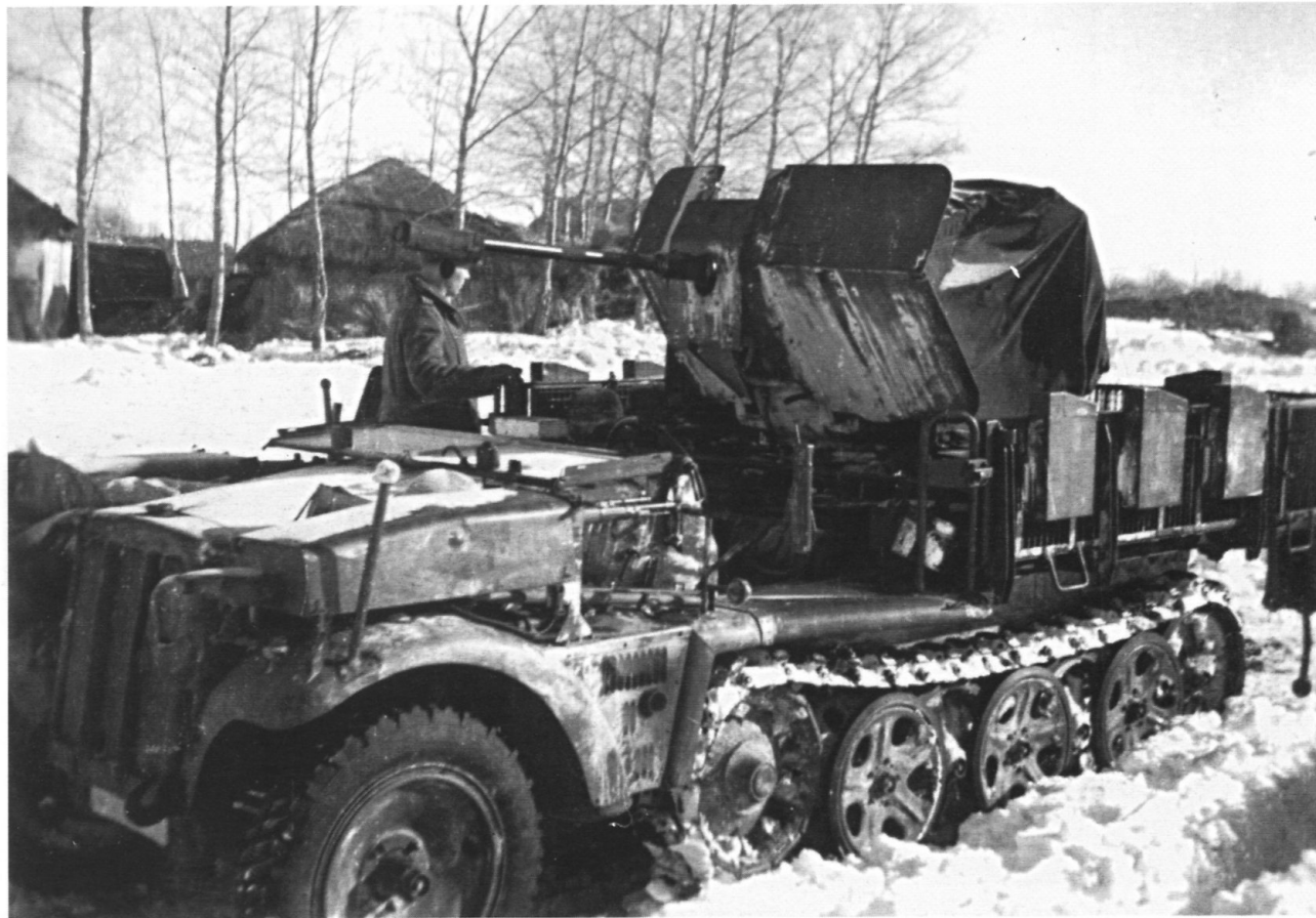
A flak gun mounted on a Sd.Kfz.7 halftrack in the winter of 1943. By the end of 1943 mechanised Waffen-SS formations had become well-equipped with flak guns. Apart from a five battery motorised flak battalion, divisions also had additional anti-aircraft platoons and companies in their Panzergrenadier, Panzer and artillery regiments.
