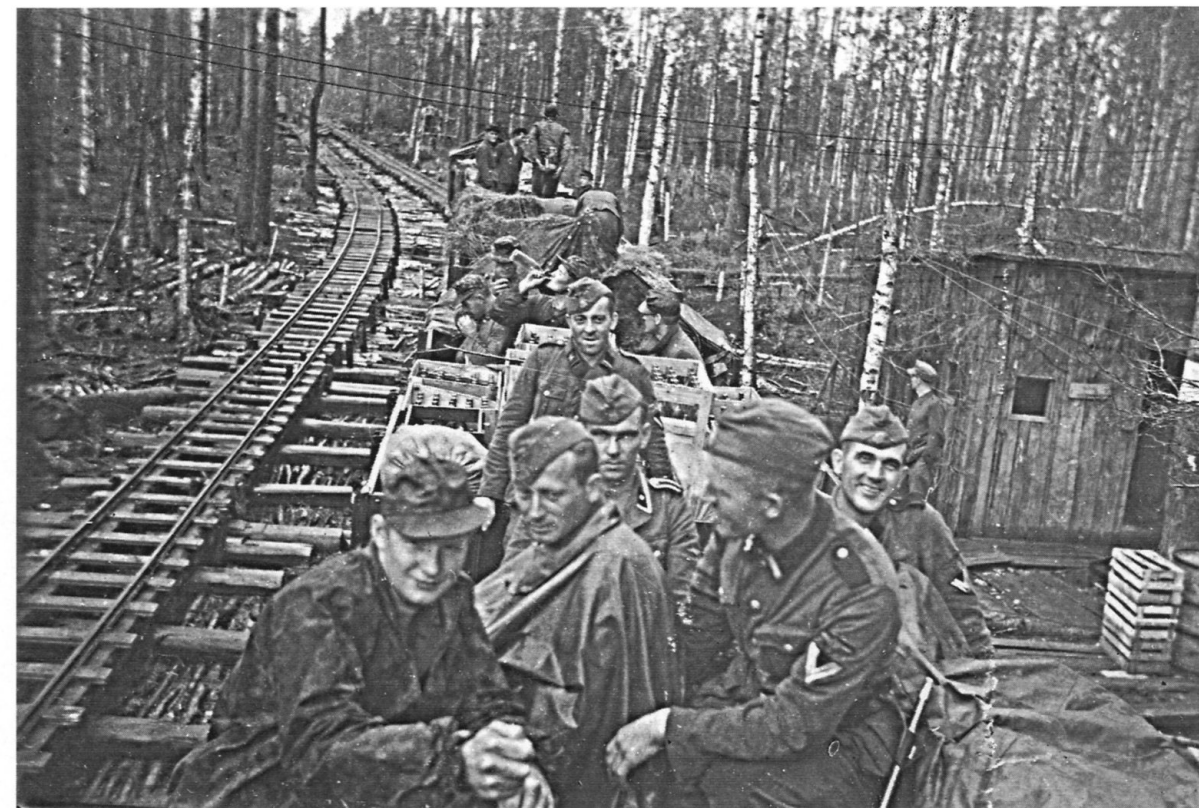
Here SS troops are making full use of the extensive narrow gauge-railroads in the East. These specially adapted flatcars were much wider in proportion to the track than wider gauge rolling stock, and could carry surprisingly heavy loads.
