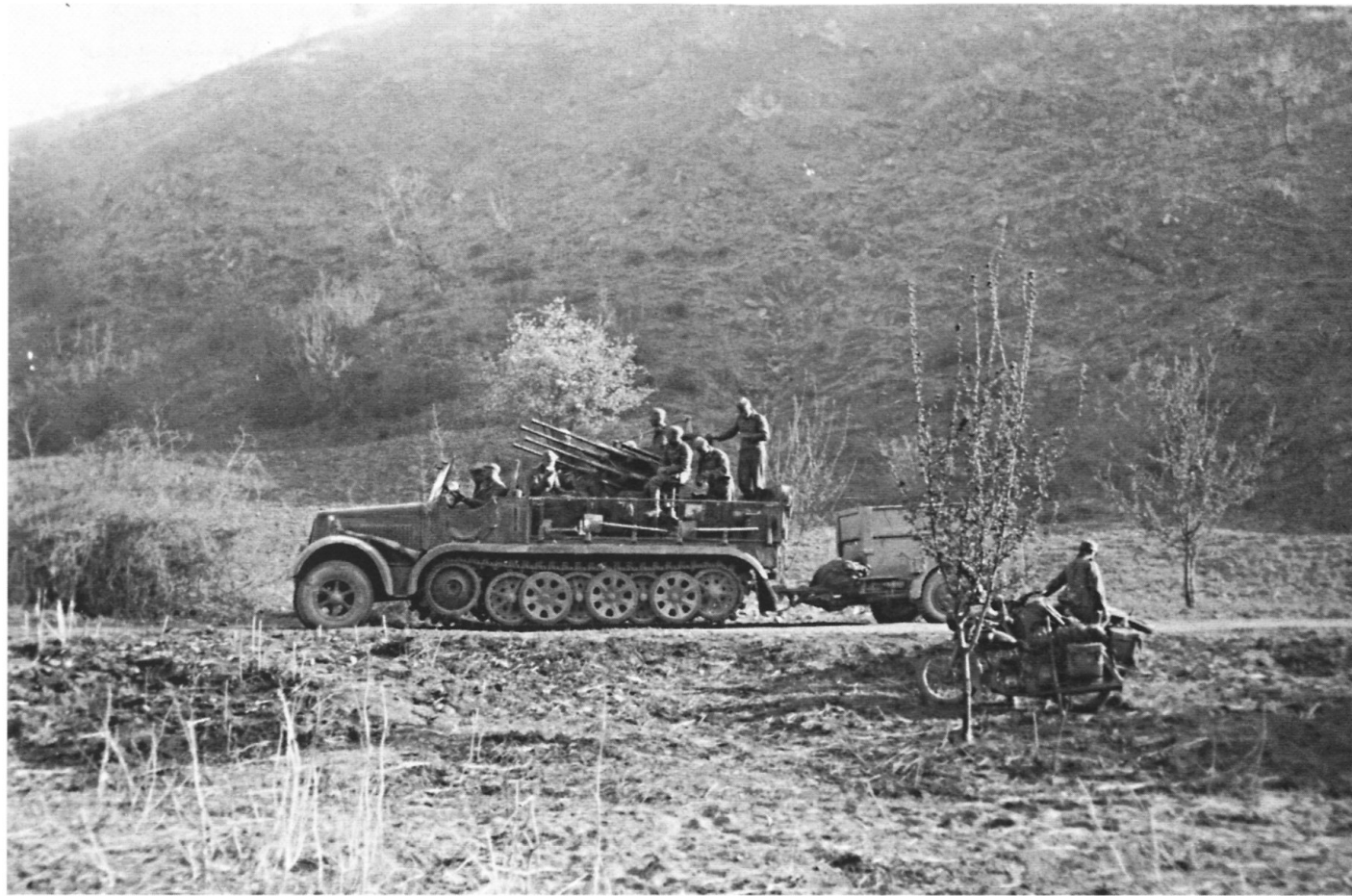
A 2cm quadruple-barrelled self-propelled anti-aircraft gun mounted on the back of a Sd.Kfz.7 halftrack advances along a road in the Balkans in October 1944. This flak unit belongs to the Prinz Eugen Division that was engaged during this time in anti-partisan duties.
