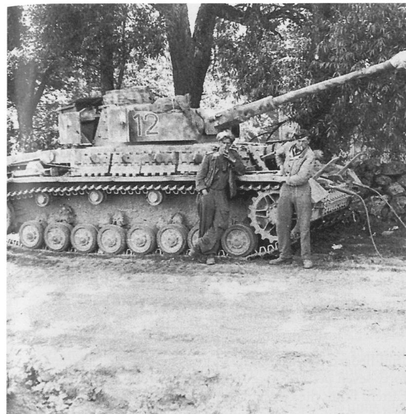
A SS tank crew take a brief respite during a lull in the fighting on the Western Front in early April 1945. The late variant Pz.Kpfw.IV has a full summer camouflage scheme. Note the spare track links that have been attached to the side of the vehicle for additional armoured protection.
