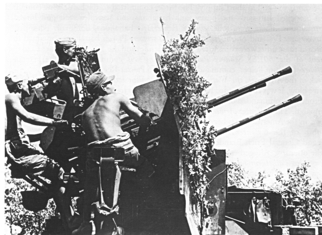
A 2cm Flakvierling 38 quadruple-barrelled self-propelled anti-aircraft gun mounted on the back of a Sd.Kfz.7 halftrack during operations in the Caen area in July 1944.
