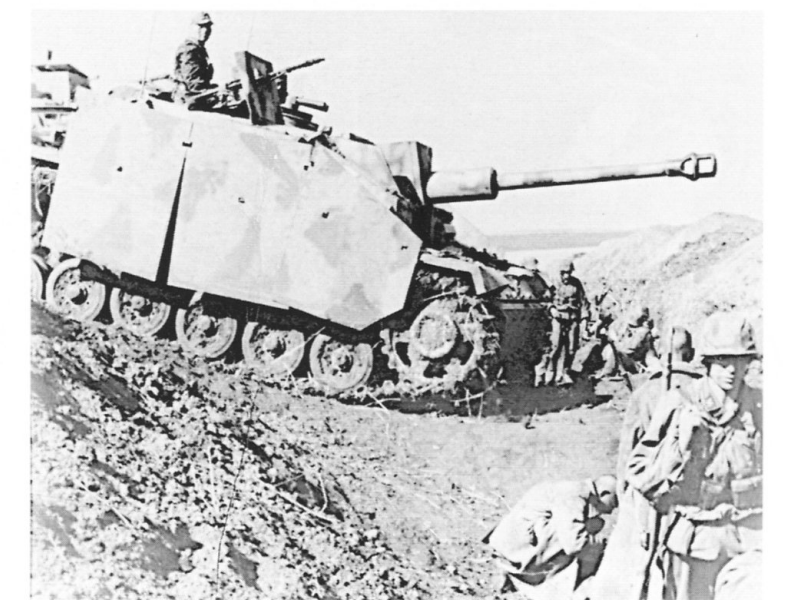
A StuG.III. Ausf.G moves forward to prepare for the final defence of Germany in March 1945. The StuG still retains its summer camouflage scheme and one of its armoured side skirts is missing, indicating that it's been lost whilst participating in fighting.
