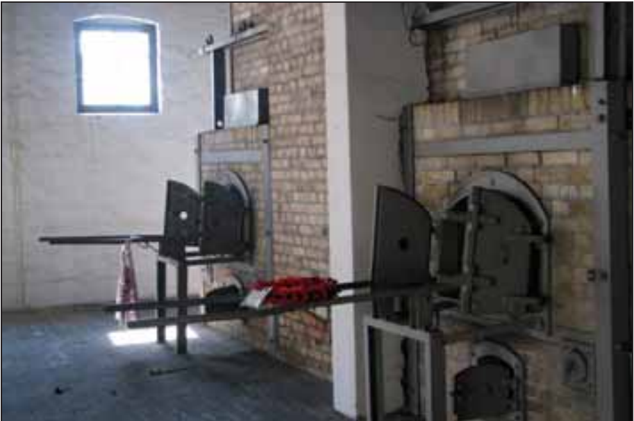
Photograph 338: KORI coke- and naphtha-fired cremation furnace at the Ravensbrück Concentration Camp. Source: http://mmlorusso.blogspot.com/2011/03/his-will-is-our-hiding-place-cont.html
