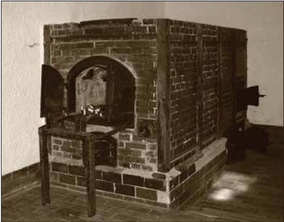
Photograph 335: KORI coke-fired cremation furnace at the Flossenbürg Camp. Source: http://commons.wikimedia.org/wiki/File:Crematory_oven_-_Flossenbürg.jpg
