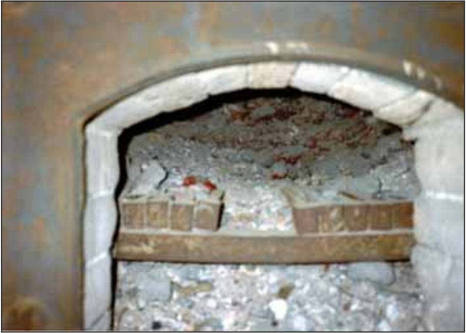
Photograph 311: The gasifier grate.
