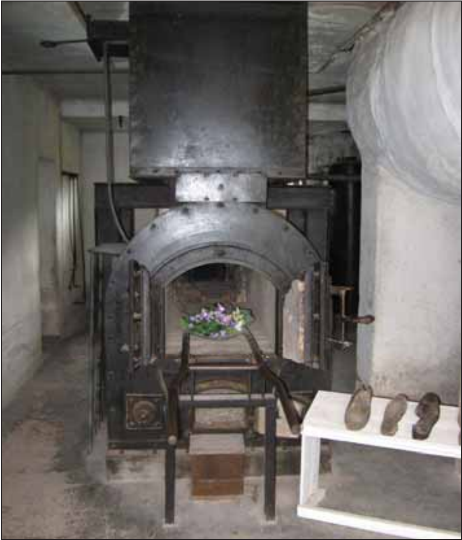
Photograph 341: KORI naphtha-fired cremation furnace at the Natzweiler-Struthof Concentration Camp. Source: http://commons.wikimedia.org/wiki/File:Natzweiler-Struthof_krematorium.JPG
