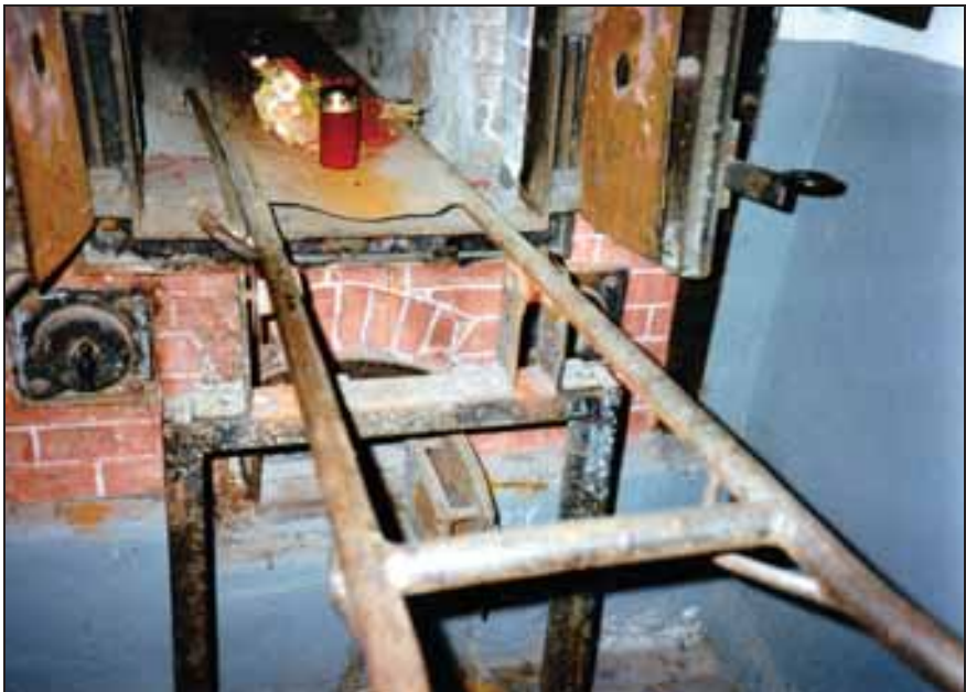
Photograph 237: as above, close-up of the corpse-introduction stretcher.
