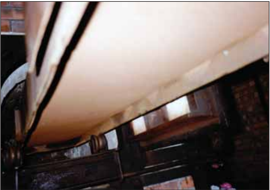
Photograph 186: Corpse-introduction cart, viewed from below. Edges of the loading stretcher running on the rollers.
