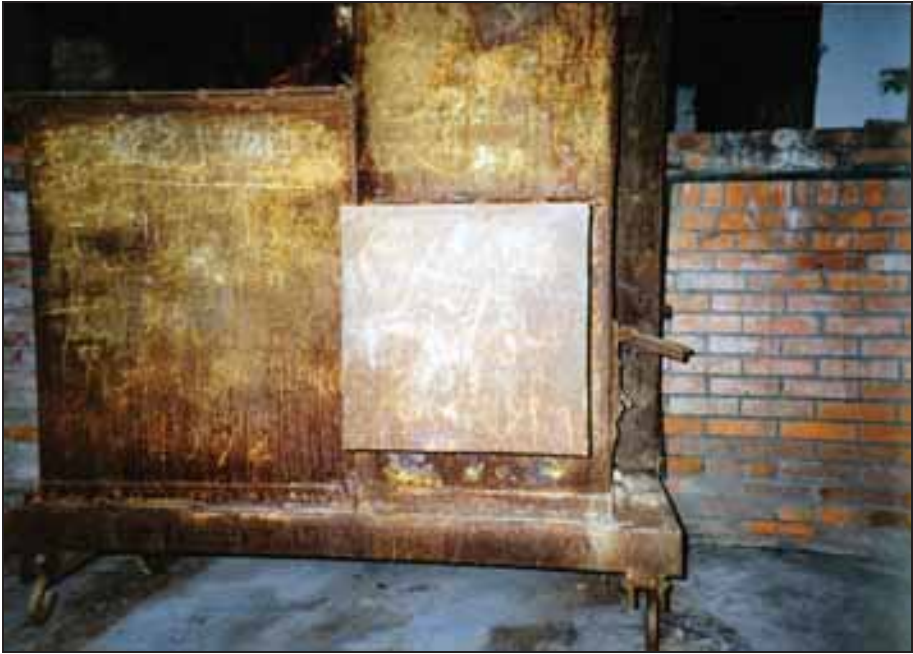
Photograph 47: Rear view of the furnace; base of the chimney with an open service door at the right-hand side. The square metal sheet welded to the chimney's bottom closes the opening for the original forced-draft blower.
