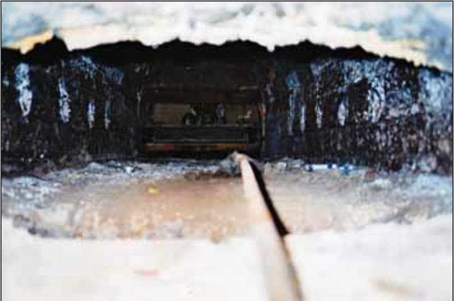
Photograph 353: as above, with the introduction cart pulled out. In the foreground, the shaft of the scraper to move cremation remains.
