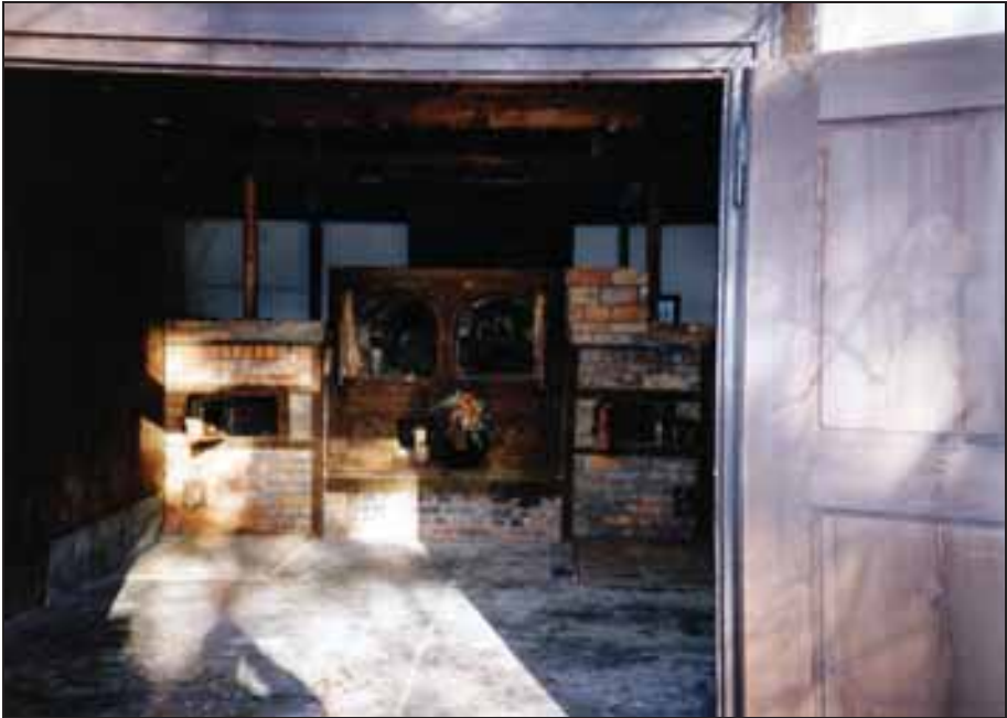
Photograph 36 (top) and 36a (bottom): Original furnace body of coated sheet metal with masonry gasifiers added to its sides.
