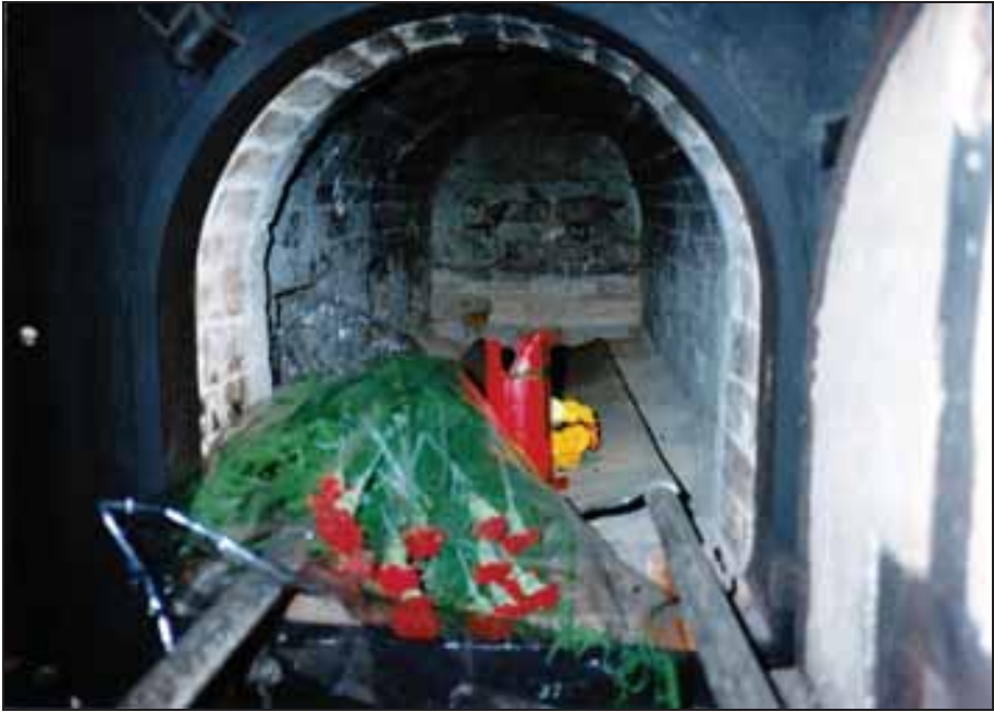
Photograph 62: Right-hand muffle; the three inter-muffle openings can be seen to the left.
