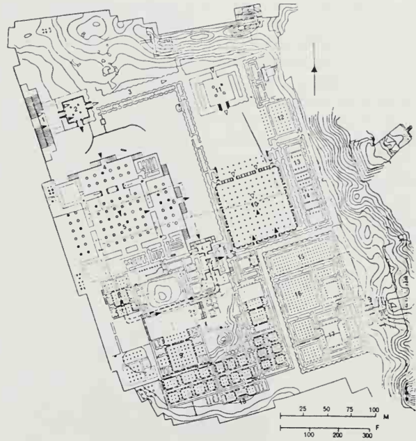
129. Plan of the Palace of Darius and Xerxes, Persepolis. 1) Great entrance stairway; 2) Gatehouse of Xerxes; 3) Audience Hall of Darius and Xerxes; 4) Throne Hall of Xerxes; 5) Palace of Darius; 6) Palace, probably rebuilt by Ataxerxes; 7) Palace of Xerxes; 8) Council Hall; 9) Restored area of the "Harem"; 10) Treasury; 11) Section of northern fortifications; 12) Royal tomb, probably of Ataxerxes
