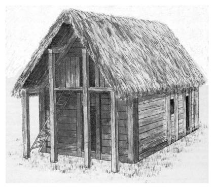
Figure 7.2 Reconstruction of a one-aisled house with roof-supporting timber-framed walls excavated at Gotland, Sweden (from Carlsson 1981).
