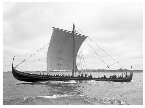
Figure 11.2 The Viking Ship Museum's reconstruction of the 60-oared longship Skuldelev 2. Built in Dublin in 1042, the ship is constructed for use in the difficult waters of the Irish Sea. It probably came to Denmark in the late 1060s or early 1070s. (Photo: Werner Karrasch, Viking Ship Museum in Roskilde.)
