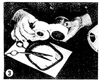
Both ends of the conister must be open. Cut a disk about I" larger in diameter from a piece of screening or a fly swatter. Hold this over one end of the conister, bend down the edge, and tope it fast
