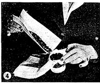
Place two handkerchiefs together and push the cloth into the canister against the screen. Pack tightly with two parts charcoal to one part soda lime and fold over the cloth. Leave wide margin all around
