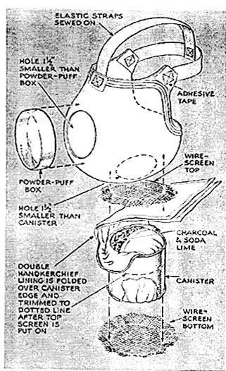
PARTS OF FINISHED MASK, and how they are assembled. The canister is kept scaled until the mask is needed. Otherwise, charcoal loses activity
