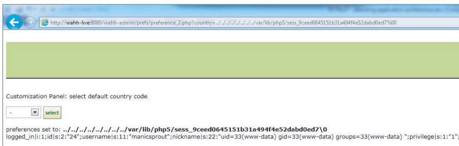
Figure 17-4: Executing the session file containing the malicious nickname via the local file inclusion function
