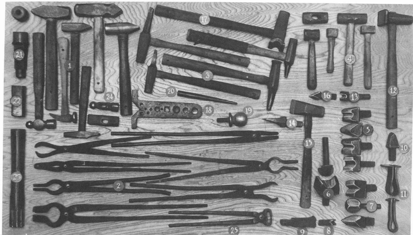
Typical blacksmith tools: 1 hammers, various weights and shapes / 2 tongs, various sizes and shapes / 3 hot punches, square- and round-ended / 4 stonecarving hammers, various weights (mild steel) / 6 cone-shaped bottom swage and matching fuller, to form blades of woodcarving gouges / 7, 8 angle-shaped swage and matching fuller, to form blades of large and small V-shaped carving gouges / 9 die to form a reinforcement rib in gouge or garden-tool blade / 11 jigs which may be clamped between vise jaws / 12 set-hammer or flatter / 14 hardy / 15 hot chisel / 17 top swage / 18 heading plate with holes of various sizes to form bolt heads (from 3/4-inch-thick scrap steel) / 19 car-hitch ball, used as forming head to shape curved blades of implements / 20 drift pin to enlarge holes started by hot punches / 21 upsetting matrix made from a section of a heavy truck axle; fits hardy hole of a large anvil / 22 squared section of a heavy truck axle from which a blacksmith hammer is to be made / 23 remnant of a heavy truck axle.
