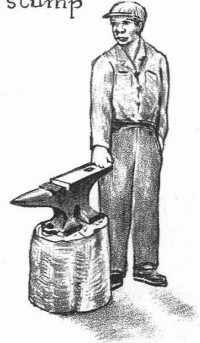
correct height of anvil on stump
